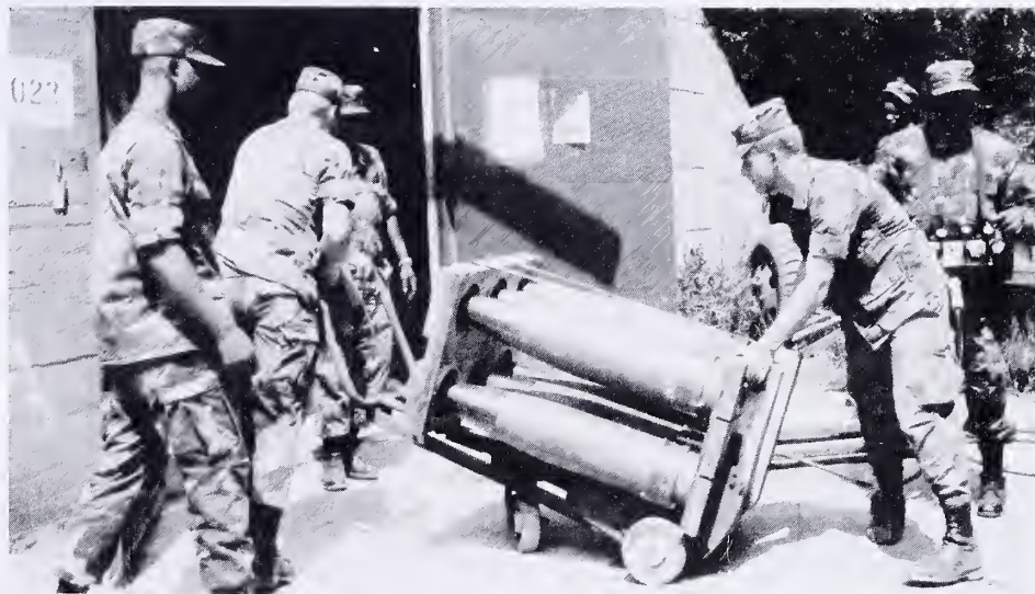
Three-wheeled handtruck is one of several basic ammo handling items engineered by the Belvoir RDE Center to upload ammunition from storage bunkers to vehicles in Europe.
